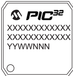
100-Lead TQFP (12x12x1 mm)
