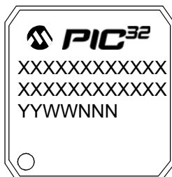
100-Lead TQFP (12x12x1 mm)
