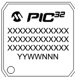
144-Lead TQFP (16x16x1 mm)
