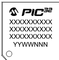
64-Lead TQFP (10x10x1 mm)
