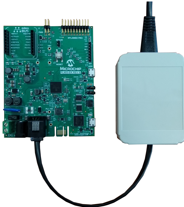
Figure 2-1. PLC-AC-Coupler accessory connected to PL485-EK
