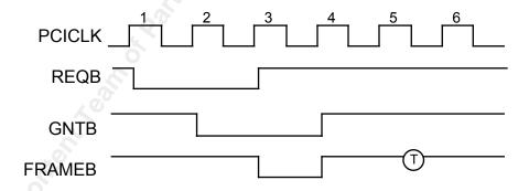
The PCI Initiator Abort Termination Diagram (Figure 38) illustrates the case when the initiator aborts a transaction on the PCI bus.
