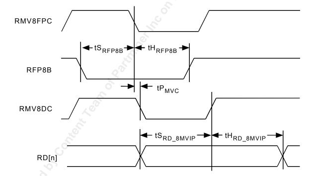
Figure 45 – Receive Data Timing (Non H-MVIP Mode)
