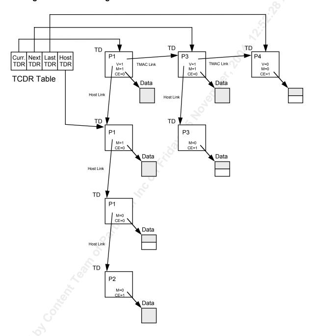
The host links the TDs vertically while the TMAC672 links TDs horizontally. Figure 15 shows the TDs for packets P1 and P2 linked by the host before the TDR is placed on the TDRR queue, as are the TDs for packet P3 and P4. Packet P3 is linked to packet P1 by the TMAC672, as is packet P4 linked to
