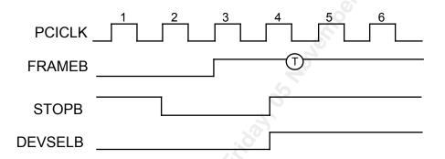
The PCI Target Abort Diagram (Figure 36) illustrates the case when the target wants to abort the current cycle. Note, when the FREEDM-32P672 is the target, it never aborts the current cycle. A target abort is an indication of a serious error and no data is transferred.
