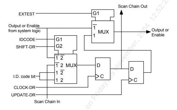
Figure 19 - Bi-directional Cell (IO\_CELL)
