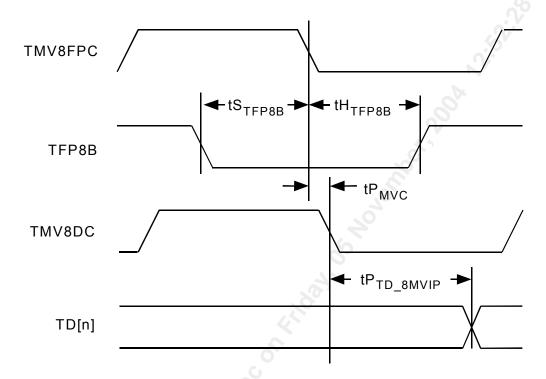
Figure 49 – Transmit Data Timing (Non H-MVIP Mode)
