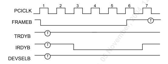
The PCI Exclusive Lock Cycle Diagram (Figure 39) illustrates the case when the current initiator locks the PCI bus. The FREEDM-32P672 will never initiate an lock, but will behave appropriately when acting as a target.
