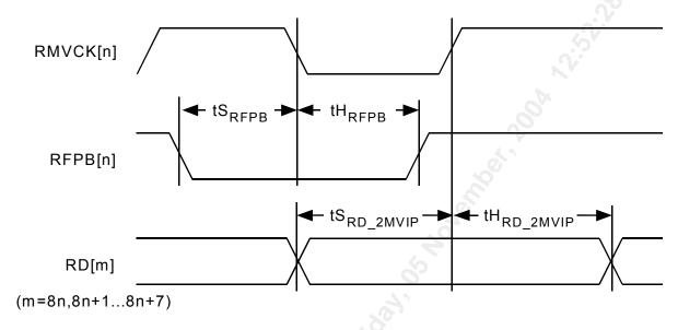
Figure 44 – Receive Data & Frame Pulse Timing (8.192 Mbps H-MVIP Mode)
