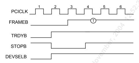
The PCI Bus Request Cycle Diagram (Figure 37) illustrates the case when the initiator is requesting the bus from the bus arbiter.
