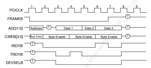
A PCI burst write transaction is shown in Figure 34. The cycle is valid for target and initiator accesses. The target is responsible for incrementing the address for the duration of the data burst. The 'T' symbol stands for a turn around cycle. A turn around cycle is required on all signals which can be driven by more than one agent.
