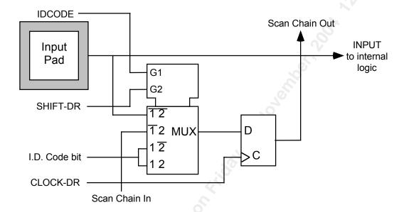
In this diagram and those that follow, CLOCK-DR is equal to TCK when the current controller state is SHIFT-DR or CAPTURE-DR, and unchanging otherwise. The multiplexor in the center of the diagram selects one of four inputs, depending on the status of select lines G1 and G2. The ID Code bit is as listed in the table above.
