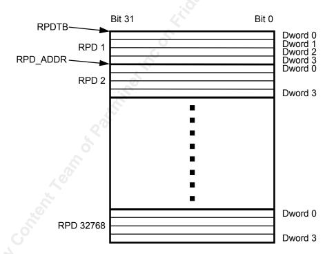
The Receive Packet Descriptor Table resides in host memory. The Rx Packet Descriptor Table Base register resides in the RMAC672; this register is initialised by the host. The RPDRs reside in host memory and are accessed using receive packet queues which are described in the next section.
