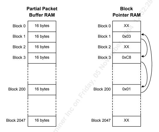
The writer and reader determine empty and full FIFO conditions using flags. Each block in the partial packet buffer has an associated flag. The writer sets the flag after the block is written and the reader clears the flag after the block is read. The flags are initialized (cleared) when the block pointers are written using indirect block writes. The reader declares a channel FIFO under-run whenever it tries to read data from a block without a set flag.
