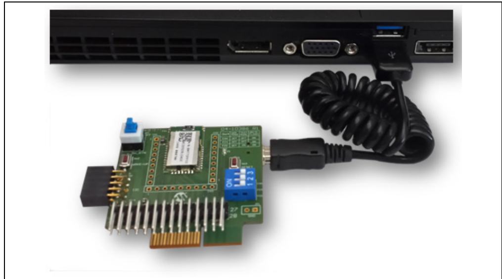
FIGURE 2-2: CONNECT THE RN4677 PICtail™ BOARD TO A HOST PC USB PORT
