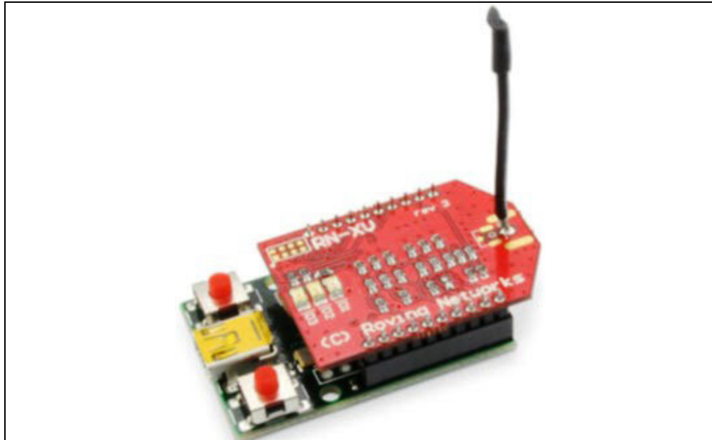
FIGURE 2-1: HARDWARE SETUP WITH RN171XV BOARD
