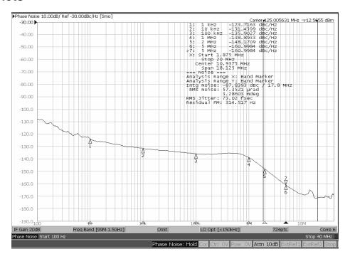
Phase Noise Plot: 125MHz, 1.875MHz - 20MHz 73fS
