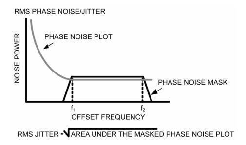
Figure 3. RMS Phase/Noise Jitter
