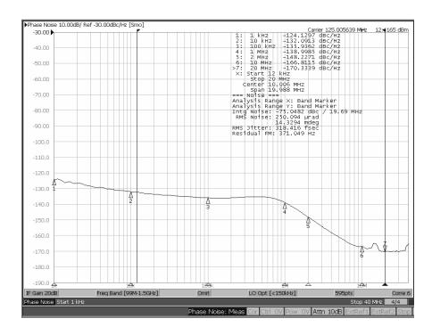
Phase Noise Plot: 125MHz, 12kHz - 20MHz 318fS
