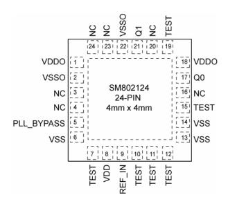
24-Pin QFN (code) (Top View)
