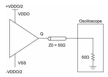
Figure 4. CMOS Output Load and Test Circuit
