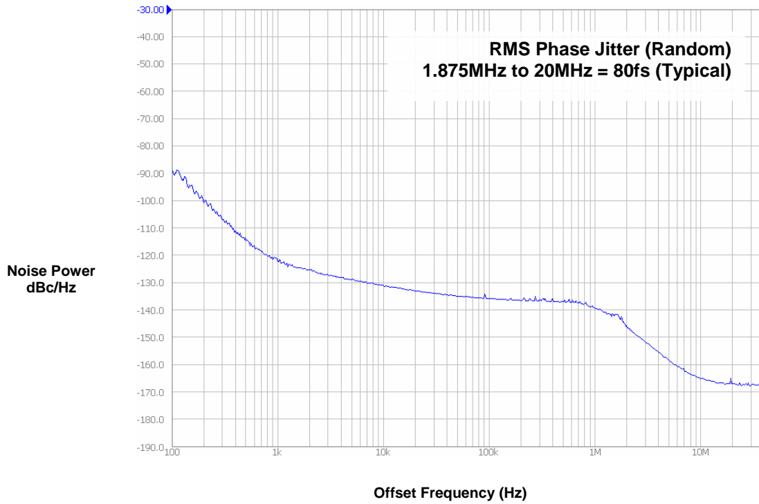
Phase Noise Plot: 156.25MHz @ 3.3V
