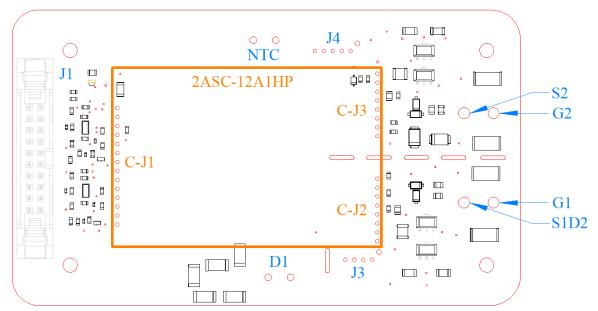
Figure 2 SP6CA1 Interconnects on Adapter Board
