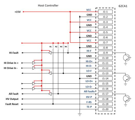
Figure 3 SP6CA1 Recommended Interface Circuitry
