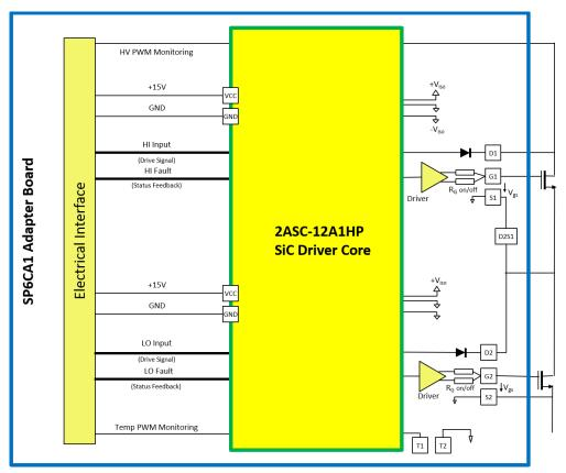
Figure 1 SP6CA1 Adapter Board Basic Topology
