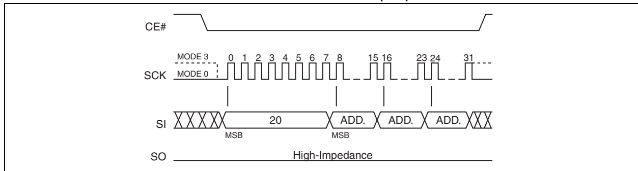
FIGURE 5-20: 4 KBYTE SECTOR-ERASE SEQUENCE (SPI)
