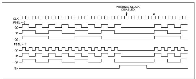
FIGURE 3-1: Timing Diagram - SY100S834L.
