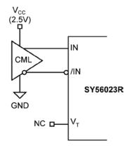
Figure 4a. CML Interface  $100\Omega$ Differential (DC-Coupled, 2.5V)
