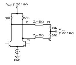
Figure 5a. 1.2V or 1.8V CML DC-Coupled Termination
