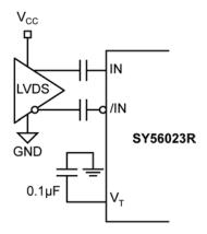
Figure 4e. LVDS Interface (AC-Coupled)
