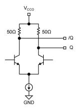
Figure 2b. Simplified CML Output Buffer
