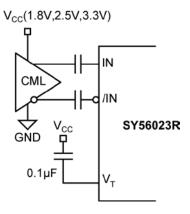
Figure 4c. CML Interface (AC-Coupled)
