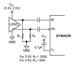
Figure 4d. LVPECL Interface (AC-Coupled)
