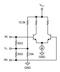
Figure 2a. Simplified Differential Input Buffer
