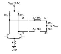
Figure 5c. CML AC-Coupled Termination V<sub>CCO</sub> 1.8V Only
