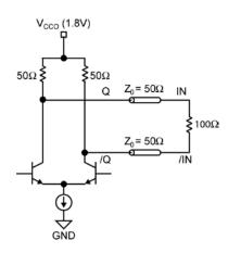
Figure 5b. 1.8V CML DC-Coupled Termination
