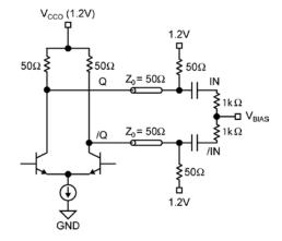
Figure 5d. CML AC-Coupled Termination  $V_{\text{CCO}}$  1.2V Only
