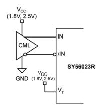
Figure 4b. CML Interface  $50\Omega$  to  $V_{CC}$ (DC-Coupled, 1.8V, 2.5V)
