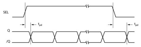
Figure 1. Propagation Delay
