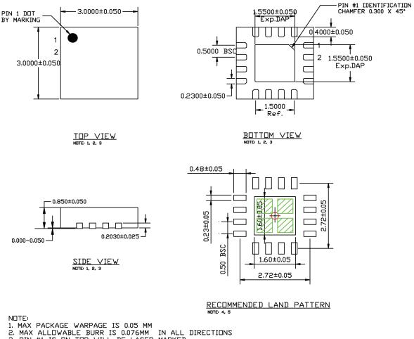
I. MAX PACKAGE WARPAGE IS 0.05 MM 2. MAX ALLOWABLE BURR IS 0.076MM IN ALL DIRECTIONS 3. PIN #1 IS ON TOP WILL BE LASER MARKED 4. RED CIRCLE IN LAND PATTERN INDICATE THERMAL VIA. SIZE SHOULD BE 0.30-0.3M IN DIAMETER AND SHOULD BE CONNECTED TO GND FOR MAX THERMAL PERFORMANCE 5. GREEN RECTANGLES (SHADED AREA) INDICATE SOLDER STENCIL OPENING ON EXPOSED PAD AREA. SIZE SHOULD BE 0.60×0.60 MM IN SIZE, 0.20 MM SPACING.
