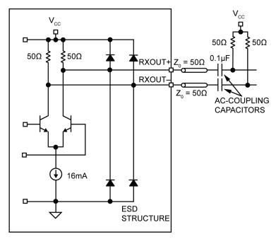
Figure 3. Typical Output Structure
