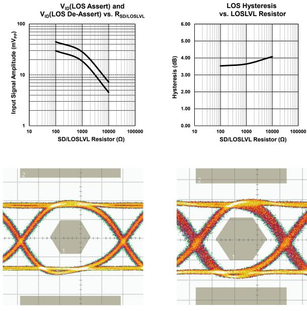
20 ps/div, Typical 10.3G Output with 10mV<sub>PP</sub> Input Signal
