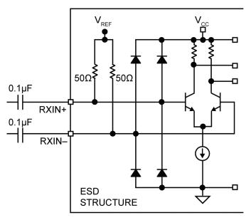
Figure 2. Typical Input Structure
