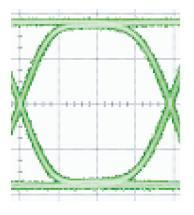
Waveform 1: Nominal Crossing Point Adjustment (50% Decision Threshold) – 20mV<sub>PP</sub> Signal Input (VTHN is tied to VTH\_REF; VTHP = 1.25V)
