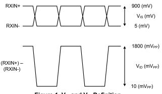
Figure 1.  $V_{\text{IS}}$  and  $V_{\text{ID}}$  Definition
