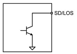
Figure 4. Typical SD/LOS Output Structure
