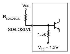
Figure 5. Typical SD/LOSLVL Setting Circuit
