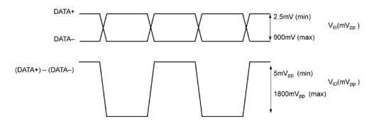
Figure 1.  $V_{\text{IS}}$  and  $V_{\text{ID}}$  Definition
