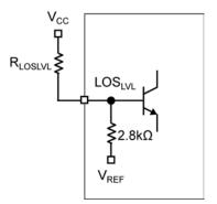
Figure 5. LOS<sub>LVL</sub> Setting Circuit
