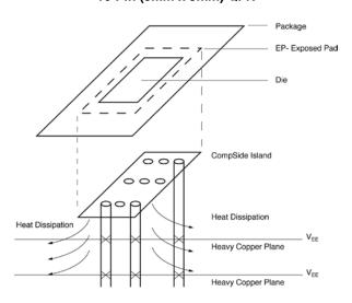
PCB Thermal Consideration for 16-Pin QFN Package
