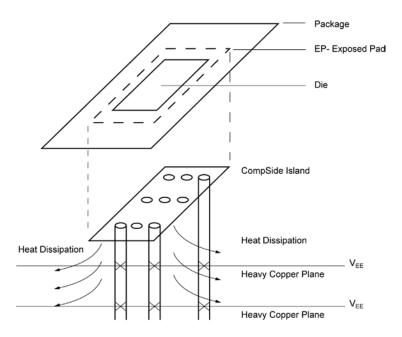
PCB Thermal Consideration for 16-Pin QFN Package
