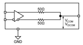
Figure 4b. LVDS Common Mode Measurement
