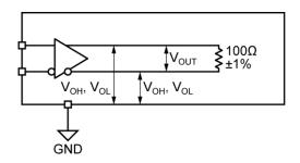
Figure 4a. LVDS Differential Measurement
