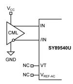
Figure 5a. LVPECL Interface (DC-Coupled)
