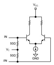
Figure 3. Simplified Differential Input Stage
