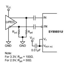
Figure 3b. LVPECL Interface (AC-Coupled)
