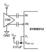
Figure 3d. CML Interface (AC-Coupled)
