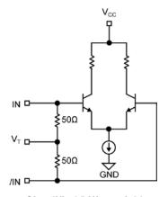
Figure 2a. Simplified Differential Input Stage
