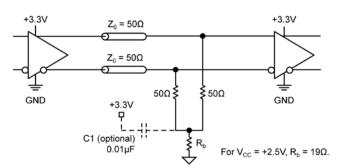
Figure 4b. Parallel Termination (3-Resistor)
