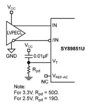
Figure 3a. LVPECL Interface (DC-Coupled)
