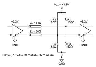
Figure 4a. Parallel Thevenin-Equivalent Termination
