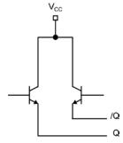
Figure 2b. Simplified LVPECL Output Stage
