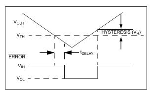
FIGURE 4-2: Error Output Operation.
