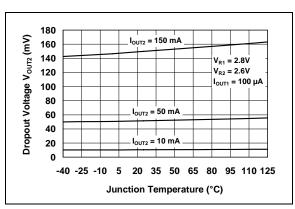
**FIGURE 2-9:** Dropout Voltage vs. Junction Temperature  $(V_{OUT2})$ .
