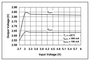
FIGURE 2-5: Output Voltage vs. Input Voltage.
