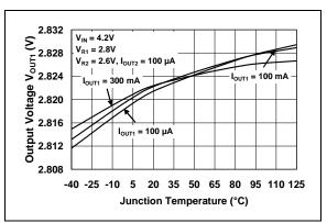
**FIGURE 2-12:** V<sub>OUT1</sub> vs. Junction Temperature.
