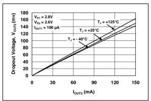
**FIGURE 2-8:** Dropout Voltage vs. Output Current (V<sub>OUT2</sub>).
