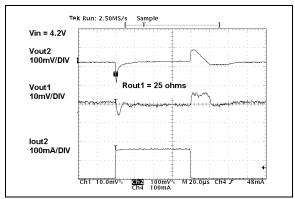
**FIGURE 2-25:** 150 mA Dynamic Load Step V<sub>OUT2</sub>.
