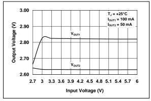
FIGURE 2-4: Output Voltage vs. Input Voltage.
