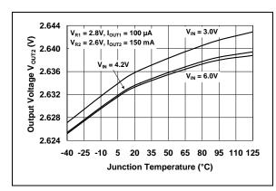
**FIGURE 2-15:** V<sub>OUT2</sub> vs. Junction Temperature.
