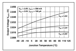
**FIGURE 2-13:** V<sub>OUT1</sub> vs. Junction Temperature.
