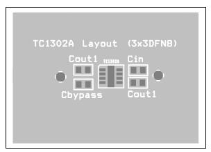
FIGURE 7-2: DFN3x3 Silk-screen Example.
