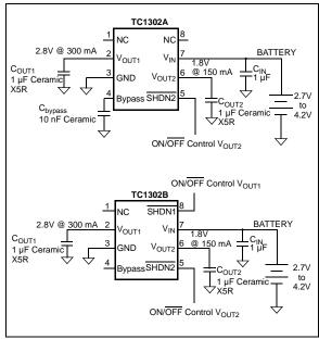
**FIGURE 6-1:** Typical Application Circuit TC1302A/B.
