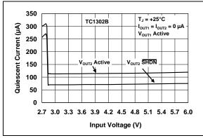
**FIGURE 2-1:** Quiescent Current vs. Input Voltage.
