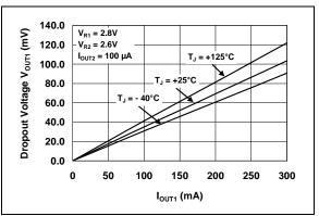
**FIGURE 2-6:** Dropout Voltage vs. Output Current (V<sub>OUT1</sub>).
