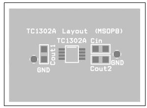
FIGURE 7-1: MSOP8 Silk-screen Layer.
