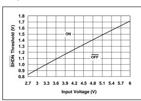
FIGURE 2-2: SHDN Voltage Threshold vs. Input Voltage.
