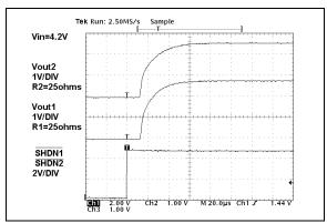
**FIGURE 2-20:**  $V_{OUT1}$  and  $V_{OUT2}$  Power-up from Shutdown TC1302B.
