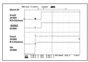
**FIGURE 2-21:** V<sub>OUT2</sub> Power-up from Shutdown Input TC1302A.
