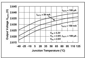
**FIGURE 2-14:** V<sub>OUT2</sub> vs. Junction Temperature.
