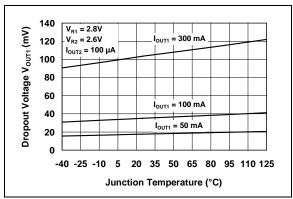
**FIGURE 2-7:** Dropout Voltage vs. Junction Temperature  $(V_{OUT1})$ .
