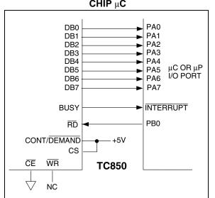
Since the PA0-PA7 inputs are dedicated to reading A/D data, the A/D CS/CE inputs can be enabled continuously. In continuous mode, data must be read in 3 bytes, as shown in Table 6-1. The required RD pulses are provided by a  $\mu$ C/ $\mu$ P output pin.
