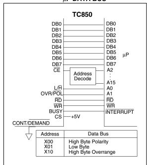
Figure 8-3 shows a typical interface to a  $\mu P$  I/O port or single-chip  $\mu C$ . The TC850 operates in the continuous mode and can either interrupt the  $\mu C/\mu P$  or be polled with an input pin.
