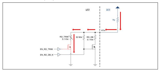
The Rd resistor presented, trimmed or untrimmed, is controlled by the CC1 and CC2 Pull-Down Values in the CC Control Register (CC\_CTL). These register fields serve the basis for the EN\_RD\_TRIM and EN\_RD\_DB\_N control signals depicted.
