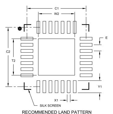
Units MILLIMETERS MAX **Dimension Limits** MIN NOM Contact Pitch 0.40 BSC Optional Center Pad Width 2.40 W2 Optional Center Pad Length T2 2.40 Contact Pad Spacing C1 3.90 Contact Pad Spacing C2 3.90
