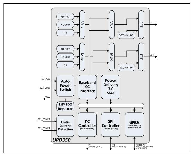
FIGURE 2-2: INTERNAL BLOCK DIAGRAM
