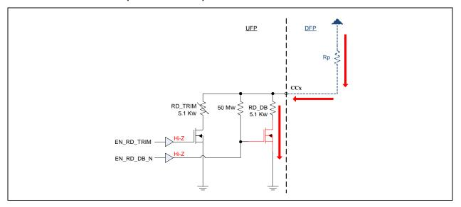
Figure 8-2 illustrates operation after the UFP has been powered over VBUS by the DFP. After the device is powered, EN\_RD\_DB asserts by default to keep the RD\_DB pull-down activated.
