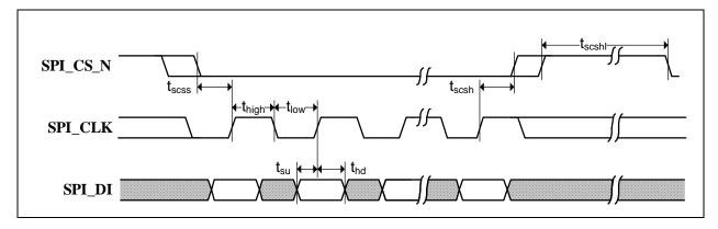
FIGURE 14-5: SPI SLAVE OUTPUT TIMING
