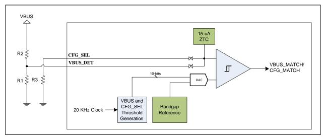
For a DFP, the VBUS comparator is useful to detect when VBUS is within the desired range per PD negotiations. This is the case when VBUS is generated by a source external to the device.
