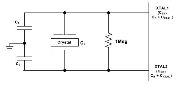
Figure 6.1 Typical Crystal Circuit
