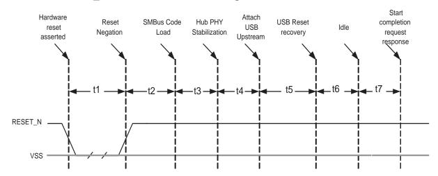
Figure 4.5 Reset\_N Timing for SMBus Mode
