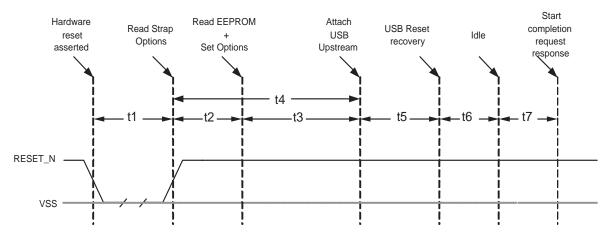
Figure 4.4 Reset\_N Timing for EEPROM Mode
