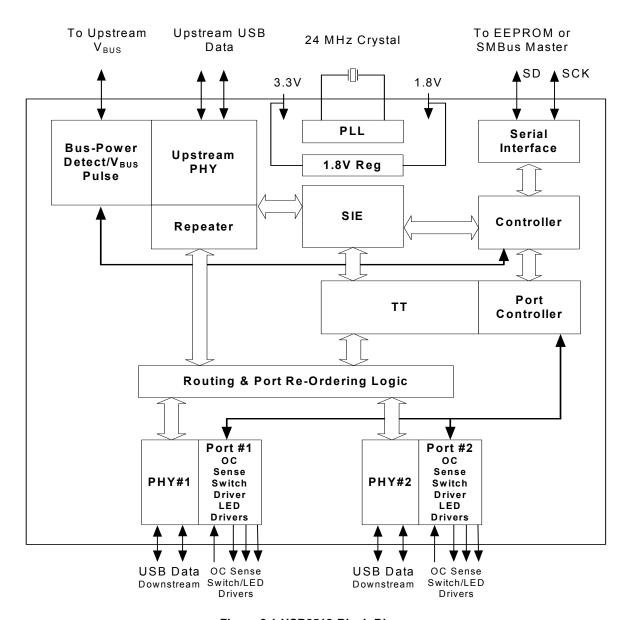
Figure 2.1 USB2512 Block Diagram
