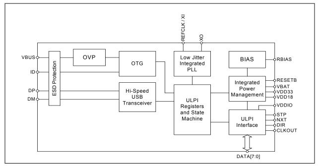
Figure 2 Block Diagram (USB3343)
