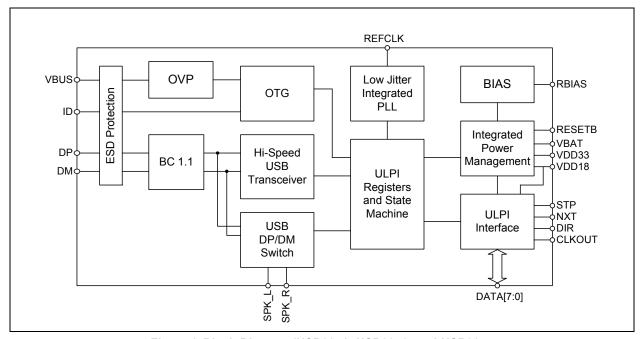
Figure 1 Block Diagram (USB3341, USB3346, and USB3347
