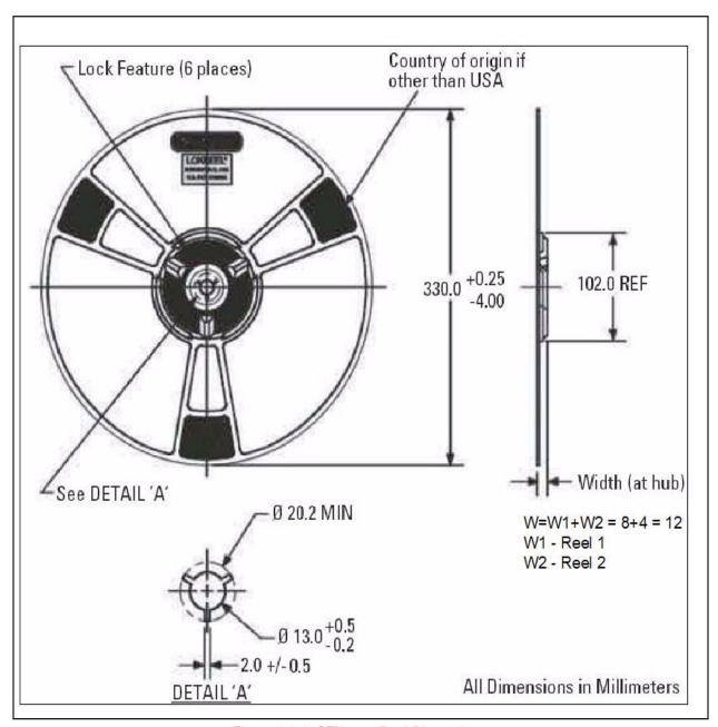
Figure 9.3 24QFN, 4x4 Reel Dimensions
