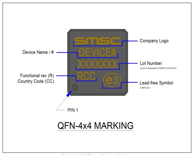
Figure 9.4 24QFN, 4x4 Package Marking
