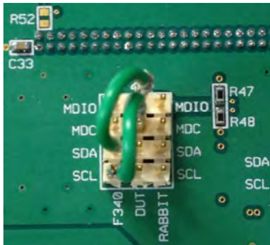
Figure 2 • MDIO/MDC Jumpers on J23 to SiLabs F340 pins
