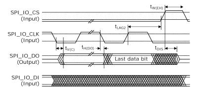
All SI signals comply with the specifications shown in the following table. The SI input timing requirements are requested at the pins of the device.
