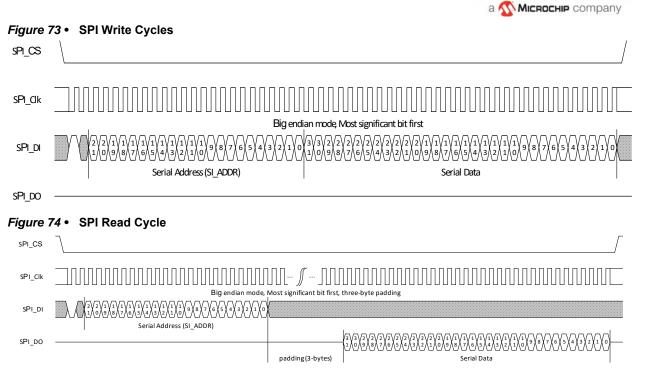
A 25 MHz SPI operating rate is used to access the CSR address space.
