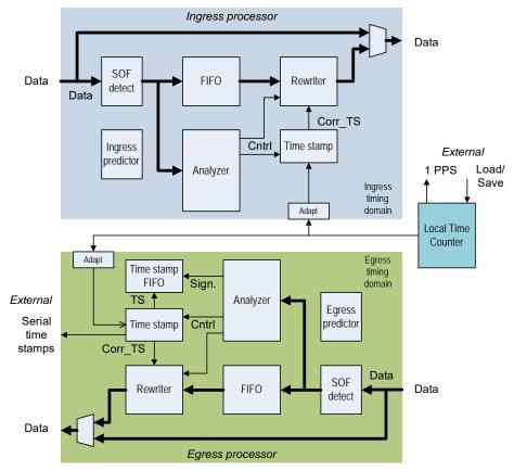
In both directions, the input data from the PHY layer is first fed to an SOF detect block. Data is then fed to both the programmable time-delay FIFO and the analyzer. The FIFO delays the data by the time needed to complete the operations necessary to update the PTP frame. That is, the data is delayed to the input of the rewriter so that the rewriter operations are known when the frame arrives. This includes the analyzer and time stamp processor block's functions.
