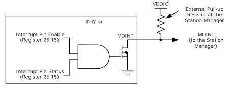
When a PHY generates an interrupt, the MDINT pin is asserted by driving low if the interrupt pin enable bit (MII register 25.15) is set.
