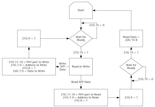
To read a value from a specific address of the two-wire serial slave device:
