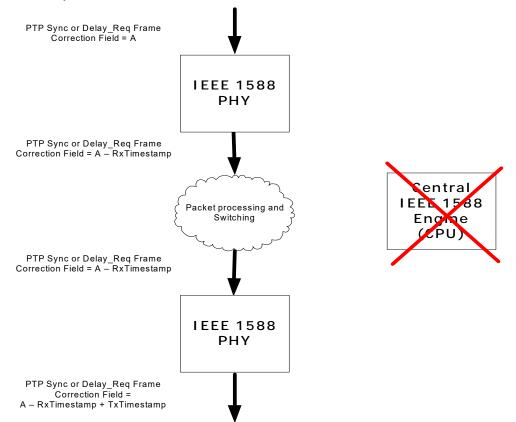
When the system works in one-step E2E TC mode Sync and Delay\_req frames must be forwarded through the system and the residence time = (Egress time stamp – Ingress time stamp) must be added to the correction field in the frame before it leaves the system.
