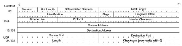
Per flow validation is performed on the Source or Destination Address in the IPv4 header. The comparator can be configured to indicate a match in the flow if the source, destination, or either the source or destination fields match.
