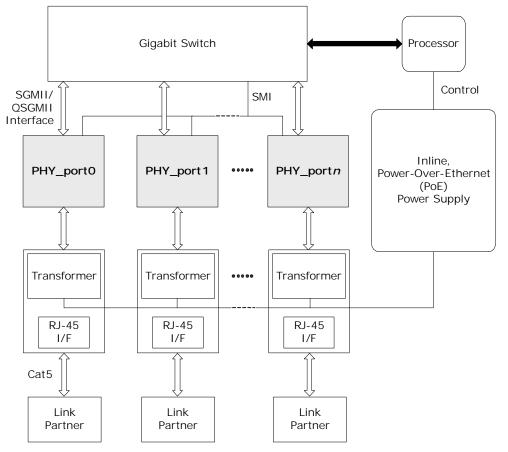
The following procedure describes the process that an Ethernet switch must perform to process inline power requests made by a link partner (LP) that is, in turn, capable of receiving inline power:
