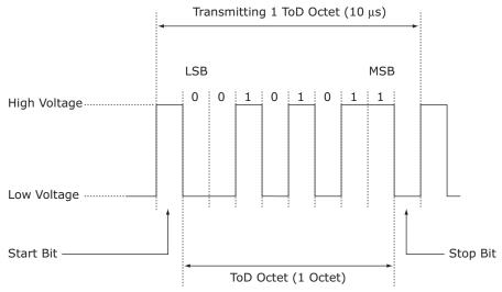
The entire Time-of-Day segment should be detected. If the second 6 octets representing the Date field are not used by the upper layer, the Date field should still be detected and its value can be ignored.
