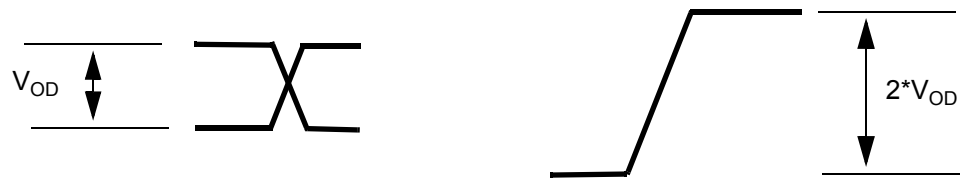
Figure 19 - Differential Voltage Parameter
