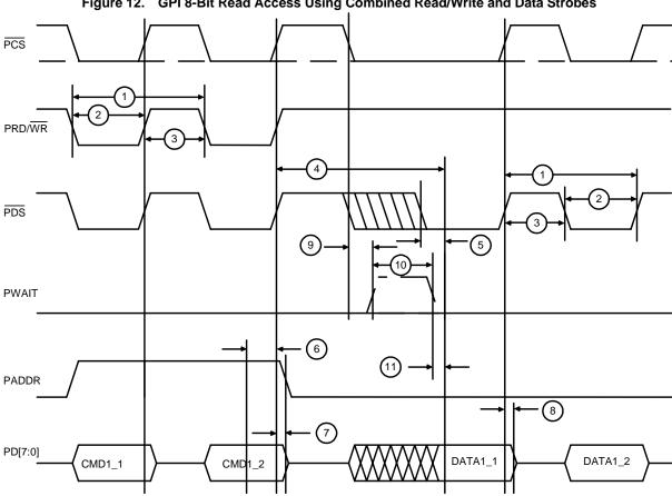
Figure 12. GPI 8-Bit Read Access Using Combined Read/Write and Data Strobes
