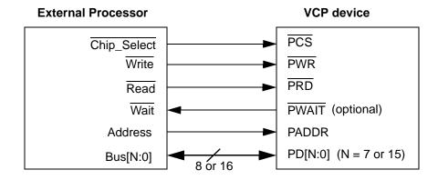
Figure 6. GPI Connections Using Combined Read/Write and Data Strobes
