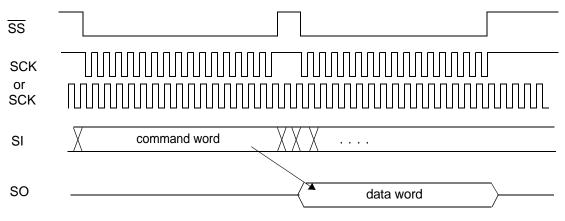
Figure 20. One Data Word Write in Byte Framing Mode with Byte Swap
