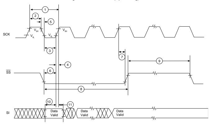
Figure 22. SPI Interface (Output Timing)
