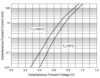
Fig. 1 - Typical Instantaneous Forward Characteristics
