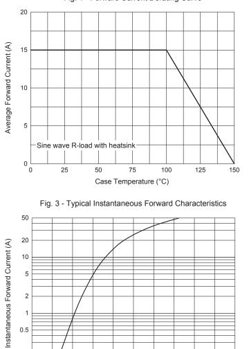
Fig. 1 - Forward Current Derating Curve
