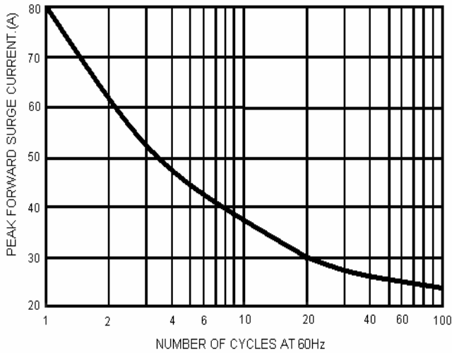
FIG.1-MAXIMUM NONO-REPETITIVE FORWARD SURGE CURRENT PER BRIDGE EELMENT
