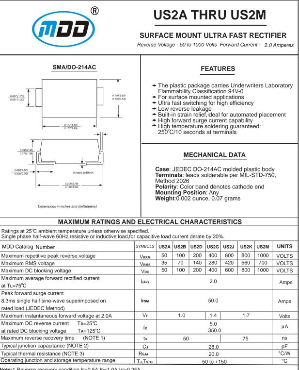
Note:1.Reverse recovery condition IF=0.5A,IR=1.0A,Irr=0.25A 2.Measured at 1MHz and applied reverse voltage of 4.0V D.C. 3.P.C.B. mounted with 0.2x0.2"(5.0x5.0mm) copper pad areas
