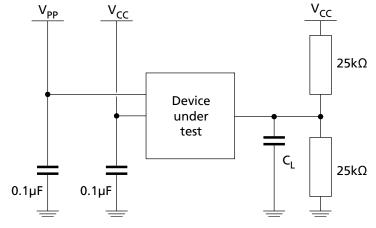
Note: 1. C<sub>L</sub> includes jig capacitance.
