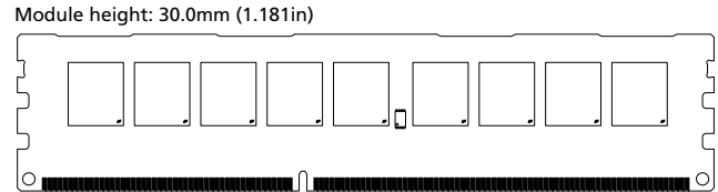
Figure 2: 240-Pin UDIMM (MO-269 R/C E3)
