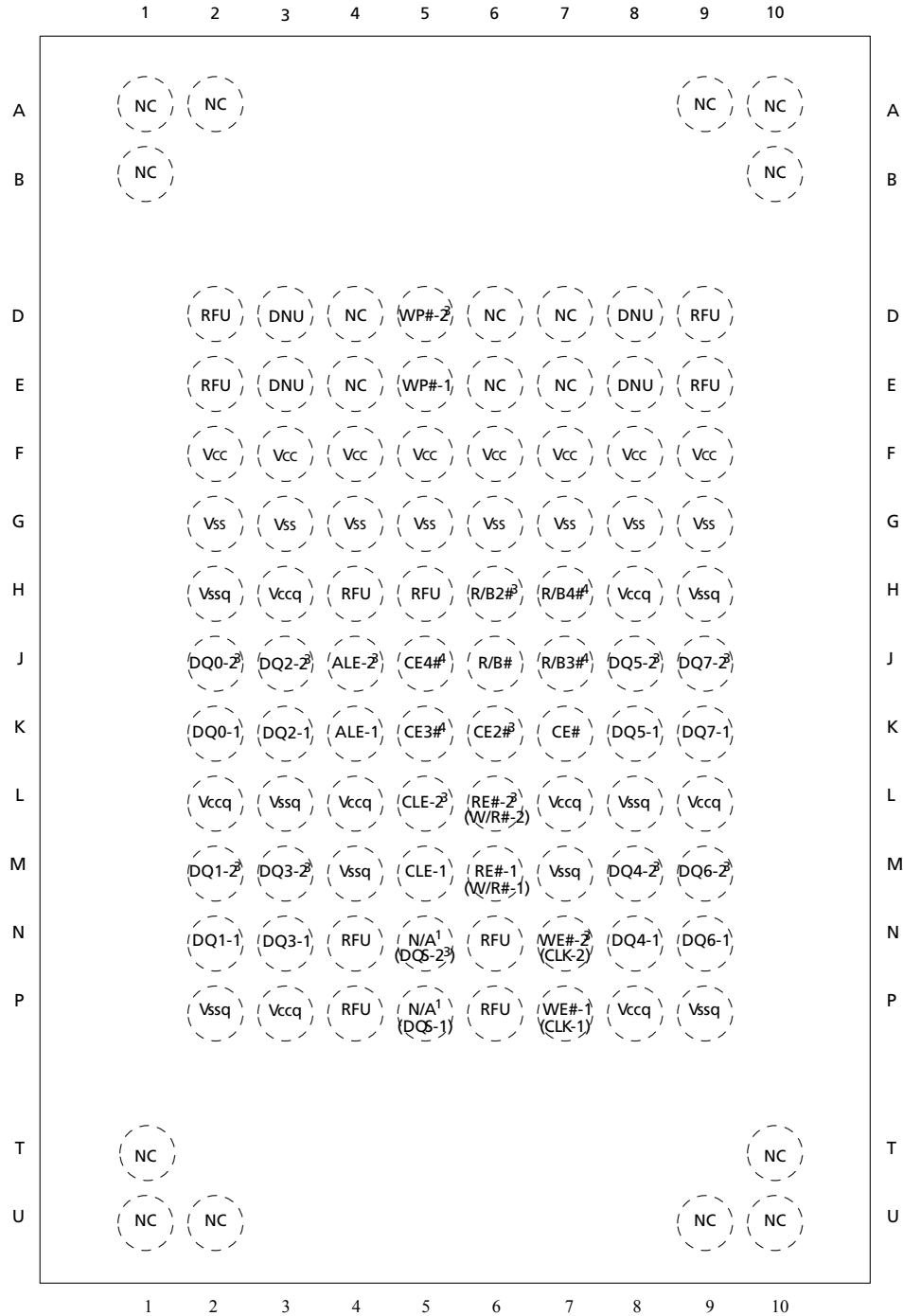
Figure 4: 100-Ball BGA (Ball-Down, Top View)
