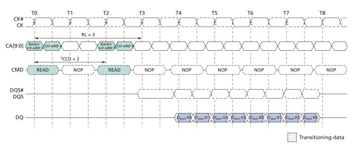
A seamless burst READ operation is supported by enabling a READ command at every other clock cycle for BL = 4 operation, every fourth clock cycle for BL = 8 operation, and
