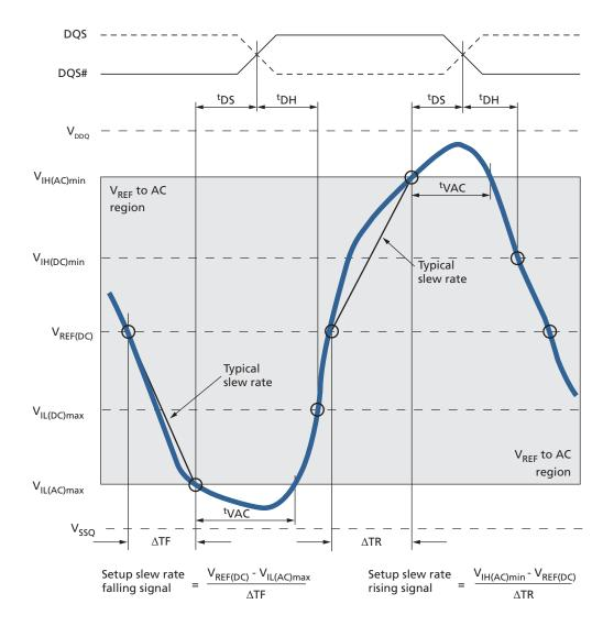
Figure 85: Typical Slew Rate - <sup>t</sup>DH for DQ Relative to Strobe
