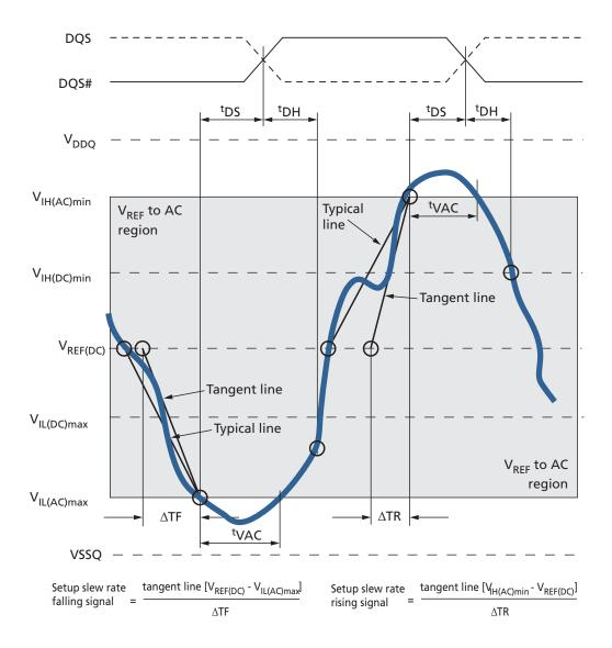
Figure 87: Tangent Line – <sup>t</sup>DH for DQ with Respect to Strobe
