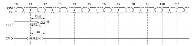
Note: 1. CKE can go LOW <sup>t</sup>IHCKE after the clock on which the REFRESH command is registered.
