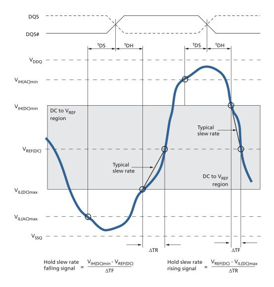
Figure 86: Tangent Line – <sup>t</sup>DS for DQ with Respect to Strobe
