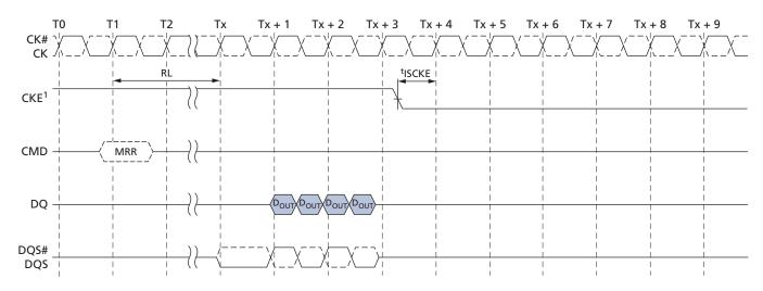
Note: 1. CKE can be registered LOW at (RL + RU(<sup>t</sup>DQSCK/<sup>t</sup>CK)+ BL/2 + 1) clock cycles after the clock on which the MRR command is registered.
