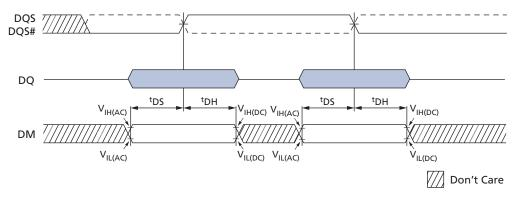
Figure 30: Write Data Mask - Second Data Bit Masked
