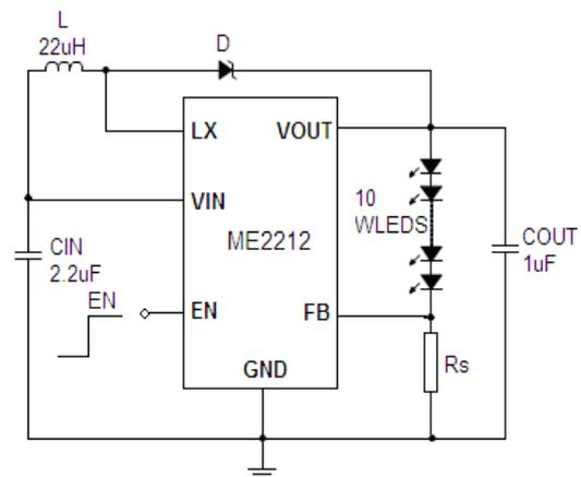
$I_{LED} = 20\text{mA}$ ,  $R_s = 10\Omega$
