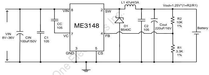
Figure 1. Constant Voltage Charge
