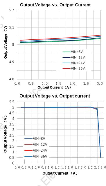
**Note:** Internal temperature compensation circuitry is provided to compensation the PCB and external line loss in system application. When the junction temperature or the output power rise, the feedback voltage will be compensated. This function is provided to compensation the PCB and external line loss in system application.
