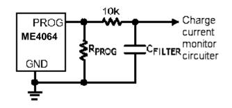
Fig.2 Isolating with capacitive load on PROG Pin
