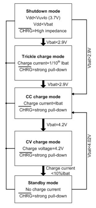
Fig.1 State diagram of a typical charge cycle
