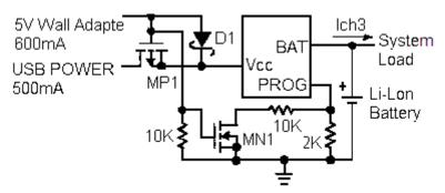
Fig.5:Combining Wall Adapter and USB Power
