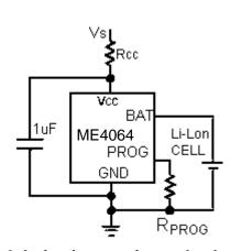
Fig.3:A circuit to maximum the thermal regulation charge current V<sub>CC</sub> bypass capacitor
