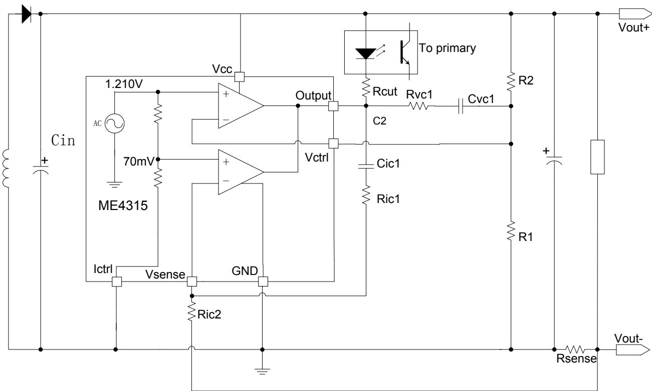
$$V_{OUT} = V_{REF} \times \frac{R1+R2}{R1} - (I_L \times R_{SS}) (V)$$
