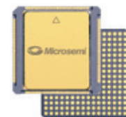
CC256 b.s. 0.67x0.67" (17.00x17.00 mm) h. 72 mils (1.847 mm) p. 7.5 mils (0.19 mm)
