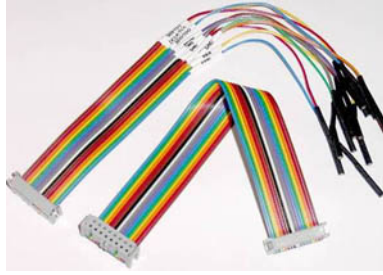
Figure 55 · Ribbon and Breakout Cables
