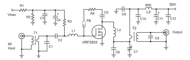
C1 1800pF ATC100B ceramic C2, C3, C5, C9, C10, C12 0.1uF 100V C6 680 pF metal clad 500V mica C7 ARCO 467 mica trimmer C8 100 pF ATC 100E ceramic C4, C11 10uF 100V Electrolytic FB small ferrite bead  $u_i$  =125 L1 20 nH 2t #18 0.188"d .2"l L2 38 nH - 2.5t #14 enam. .25" dia.
