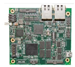
The SBC1651 is ideal for high-performance. low-power embedded applications. Freescale's i.MX515 ARM Cortex-A8 CPU operates at 800MHz delivering the performance needed to run multimedia-rich applications in embedded environments. Offering several embedded I/O features, the SBC1651 also consumes minimal power, satisfying the demanding environmental conditions in which OEMs must operate.
