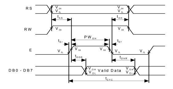
Fig.2 Read Operation Timing
