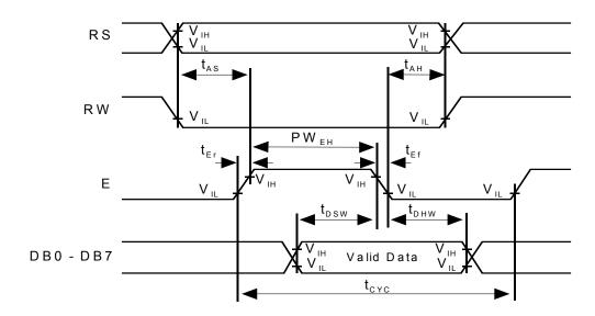
**Fig.1 Write Operation Timing**
