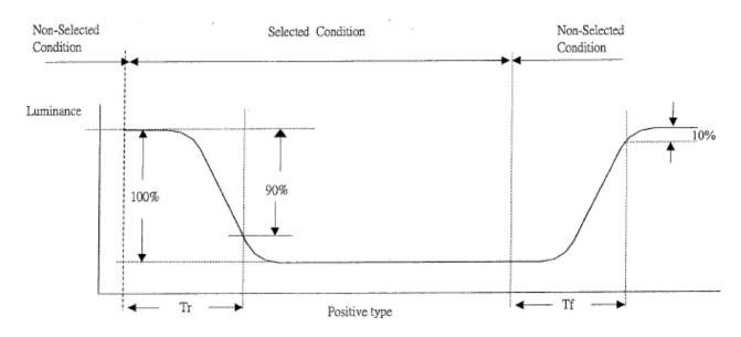
Electro - Optical Characteristics are measured by
