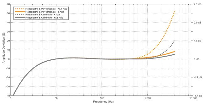
The piezoelectric accelerometer sampled at 20kHz with a 5 kHz filter. Adequate compression of the tape was achieved by first bolting the unit to allow the tape to set, then removing the bolts. The mounting torque of these bolts was 70 in-oz.
