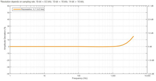
Note that the Piezoresistive accelerometer has a DC response (can measure down to 0 hertz). The plot only goes to 1 Hz because it is on a logarithmic scale. The piezoresistive accelerometer sampled at 20kHz with a 5 kHz filter. The unit was bolted down with a mounting torque of 100 in-oz.
