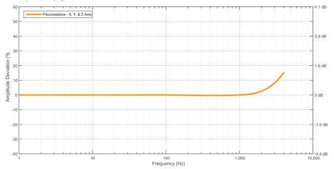
Note that the Piezoresistive accelerometer has a DC response (can measure down to 0 hertz). The plot only goes to 1 Hz because it is on a logarithmic scale. The piezoresistive accelerometer sampled at 20kHz with a 5 kHz filter. The unit was bolted down with a mounting torque of 100 in-oz.
