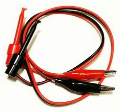
Figure 59: Simple alligator clips and/or IC hooks can be used for quick and simple testing. These are not advisable as long term connection solutions.
